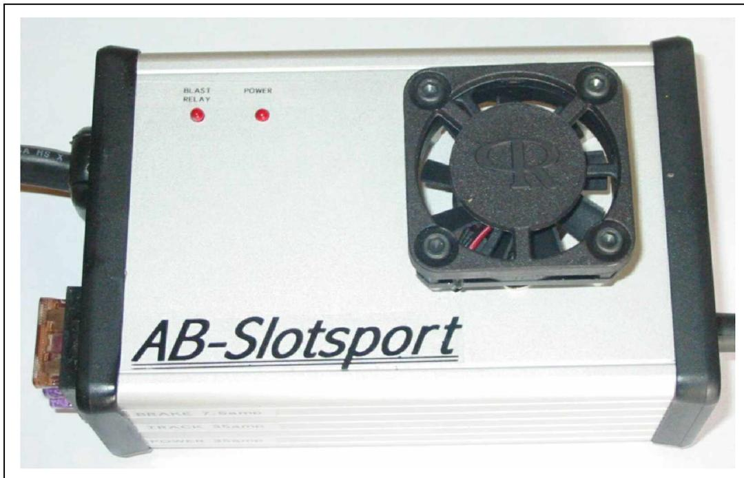
The fan should sit directly over the transistor as shown in the picture. You will need to seat the fan on 4 small threaded spacers in order for the fan blades to clear the top of the transistor.
