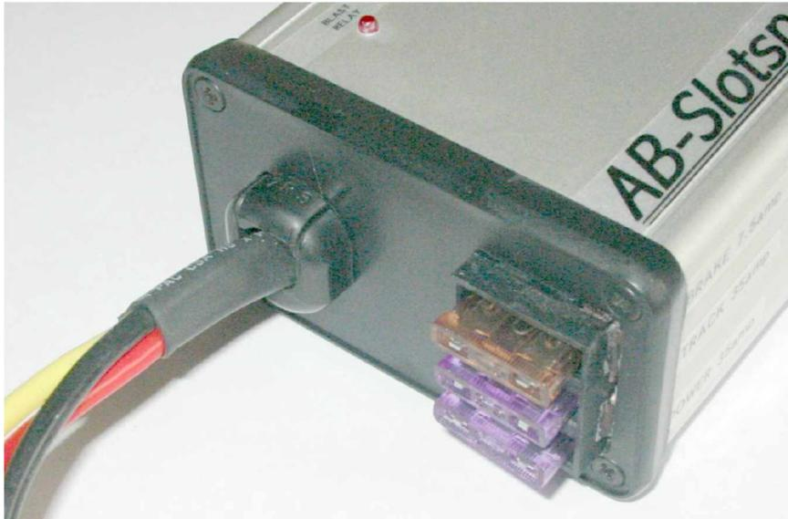
It can be an idea to fit the fuses as a “block” through the end cover plate. This makes the fuses accessible and also acts as a “terminal block for soldering wires inside the box.
