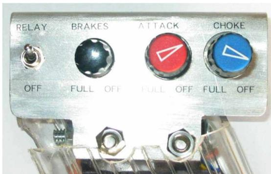
The bracket may be bolted to the rear of the controller frame. For racers racing on scale track, the blast relay switch option is a good idea, so you can switch out the blast relay to “quieten” frisky cars on tight tracks.
